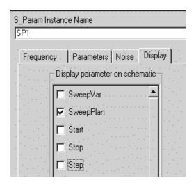
S-parameter simulation controller set to assign FREQ to be the sweep plan values.
