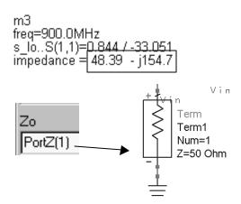
c. Change the Zo setting to PortZ(1) as shown and you will get the same answer as setting Zo to 50. However, if you did have a different port impedance (for example Z=75 Ohm) then the PortZ setting would calculate the readout using 75.
