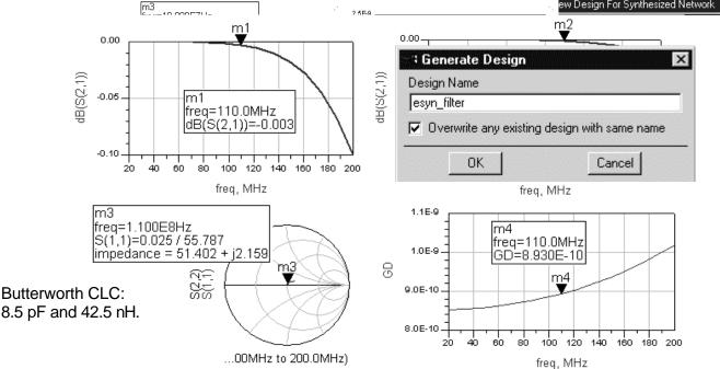
go back to the schematic window (filter \_esyn) and click: Tools > E-syn > Place New Design For Synthesized Network – this menu command only appears after synthesis. A dialog box will appear for you to name the filter. Type in a name and click OK.
