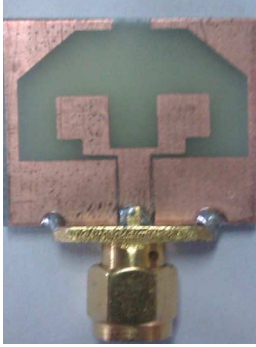
Fig. 2. Photograph of the fabricated compact UWB microstrip antenna.
