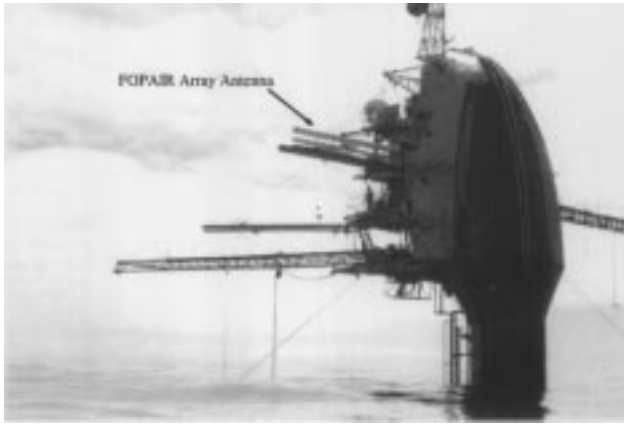
Fig. 1. FOPAIR configuration on the R/P FLIP during the marine boundary layer experiment.
