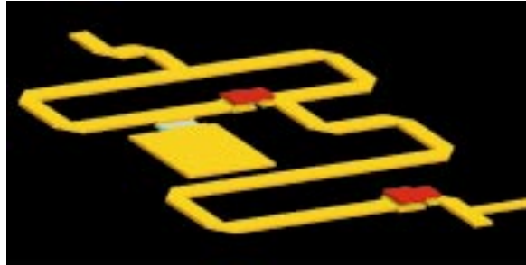
Microstrip traces and circuit elements
